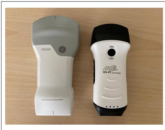
**Figure 1.** Wireless ultrasound probes used in this study (V-Scan, GE, on the left; Cerbero, ATL Milano, on the right). Both devices are provided with both a linear transducer (for venipuncture) and a convex transducer (for tip location).
